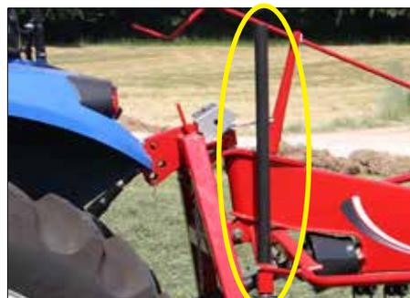
The jack stand is mounted on the main frame.
