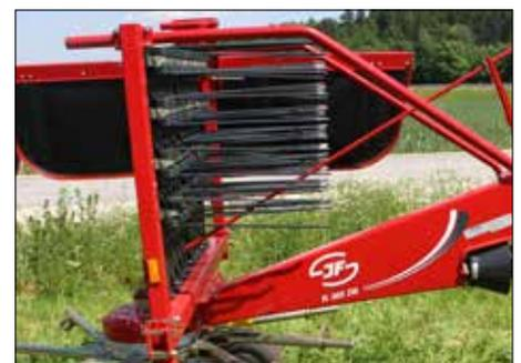
The tine arms are safely placed onto the tine arm carrier.
