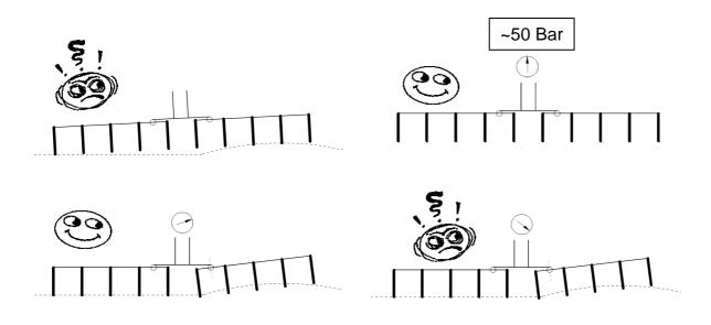
Setting the accumulator pressure is done by pulling the tractors hydraulic lever that is used to unfold Delta Flex. When unfolded, the value on the pressure gauge will increase. Setting a value of about 60 bar should result in the correct 50 bars when working in the field.
