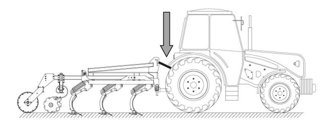
The top link must never be horizontal or parallel to the lower linkages as the cultivator will run unsteadily and make the steering of the tractor difficult.
