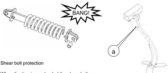
When the tine is overloaded the shear bolt snaps. The broken shearbolt (a) must be replaced by a new shearbolt (DIN 931 quality 10,9).
