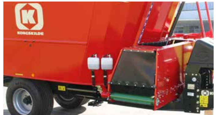
The B range for professional discharge with cross conveyor at front – VM-SB and VM-B, and one side elevator option.
