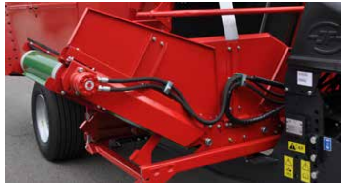
The X-range - the flexible 4-in-one cross conveyor belt solution (flat – side shift – elevator right and left) – VM-SB X and VM-B X.
