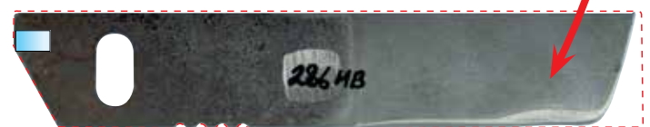
High-strength steel (S650) after the test
