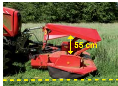
Contour Float - even ground following
