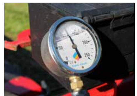
A Manometer shows the ground pressure
