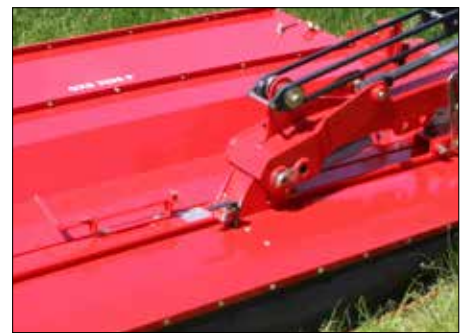
The GXS-machines have centre suspension which ensures good ground adaptation
