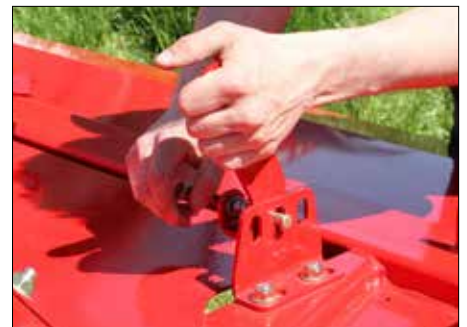
Adjustment of the degree of conditioning on the PE-conditioner is made without tools!
