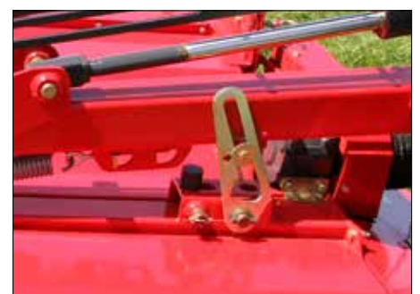
Automatic transport safety device
