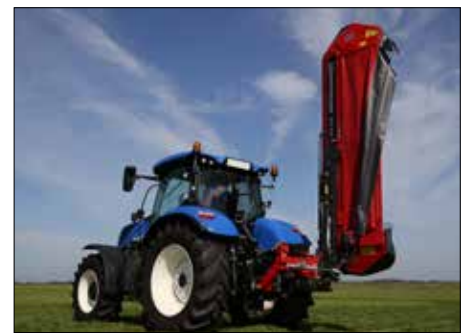
Standard transport position
