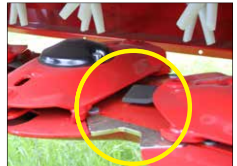
The counter knife is 2 mm higher than the cover of the cutter bar
