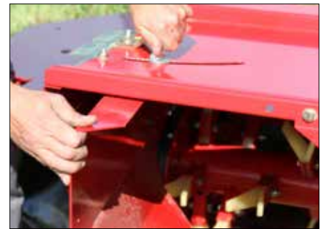
Adjustment of conditioner plate
