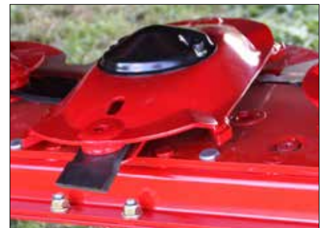
Q+ disc with twisted Q+ blades
