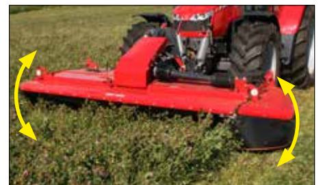
Flexible headstock for perfect ground contour following.
