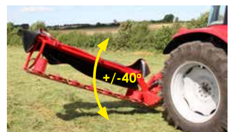
The machine can also work on slopes and along ditches and dikes with inclinations of up to +/- 40 degrees!
