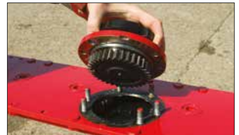
The Top Service design of the cutter bar makes it possible to check and replace a gear wheel or bearing on each disc.
