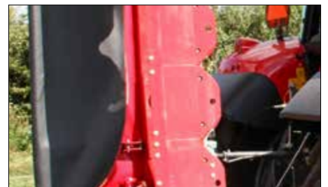
Full-covering skids that protect the gearbox from underneath.
